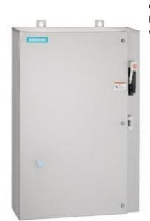
Non-reversing motor starter Size 0 Three phase full voltage Solidstate overload relay OLRelay amp range 0.25-1A 208VAC 60HZ coil Combination type 30Amp fusible disconnect 30 Amp /600V fuse clip Encl NEMA type 4X 316 S-steel Water/dust tight non-corrosive Extrawide enclosure
