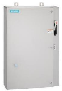
Non-reversing motor starter Size 0 Three phase full voltage Solidstate overload relay OLRelay amp range 0.25-1A 208VAC 60HZ coil Combination type 30Amp non-fusible disconnect Encl NEMA type 4X 316 S-steel Water/dust tight non-corrosive Extra-wide enclosure
