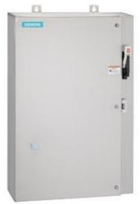
Non-reversing motor starter Size 0 Three phase full voltage Solidstate overload relay OLRelay amp range 0.25-1A 110VAC 50HZ / 120VAC 60HZ coil Combination type 30Amp non-fusible disconnect Encl NEMA type 4X 316 S-steel Water/dust tight non-corrosive Extrawide enclosure
