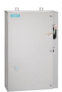
Non-reversing motor starter Size 0 Three phase full voltage Solidstate overload relay OLRelay amp range 0.25-1A 240VAC 50HZ / 277VAC 60HZ coil Combination type 30Amp fusible disconnect 30 Amp /600V fuse clip Encl NEMA type 4X 316 S-steel Water/dust tight non-corrosive Extra-wide enclosure
