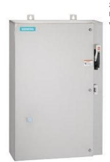
Non-reversing motor starter Size 0 Three phase full voltage Solidstate overload relay OLRelay amp range 0.25-1A 240VAC 50HZ / 277VAC 60HZ coil Combination type 30Amp non-fusible disconnect Encl NEMA type 4X 316 S-steel Water/dust tight non-corrosive Extrawide enclosure
