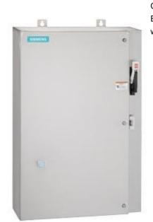
Non-reversing motor starter Size 0 Three phase full voltage Solidstate overload relay OLRelay amp range 0.25-1A 24Vdc coil Combination type 30Amp fusible disconnect 30 Amp /600V fuse clip Encl NEMA type 4X 316 S-steel Water/dust tight non-corrosive Extrawide enclosure
