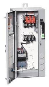
Non-reversing motor starter Size 0 Three phase full voltage Solidstate overload relay OLRelay amp range 0.25-1A 24Vdc coil Combination type 30Amp fusible disconnect 30 Amp /600V fuse clip Enclosure NEMA type 4/12 Water/dust tight weather proof Standard width enclosure
