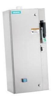
Non-reversing motor starter Size 0 Three phase full voltage Solidstate overload relay OLRelay amp range 0.25-1A 24Vdc coil Combination type 30Amp fusible disconnect 30Amp / 250V fuse clip Encl NEMA type 4X 304 S-steel Water/dust tight non-corrosive Standard width enclosure
