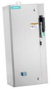
Non-reversing motor starter Size 0 Three phase full voltage Solidstate overload relay OLRelay amp range 0.25-1A 24Vdc coil Combination type 30Amp non-fusible disconnect Encl NEMA type 4X 304 S-steel Water/dust tight non-corrosive Standard width enclosure
