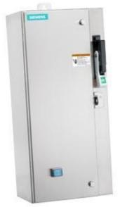
Non-reversing motor starter Size 0 Three phase full voltage Solidstate overload relay OLRelay amp range 0.25-1A Combination type 30Amp fusible disconnect 30 Amp /600V fuse clip Encl NEMA type 4X 316 S-steel Water/dust tight non-corrosive Standard width enclosure
