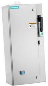
Non-reversing motor starter Size 0 Three phase full voltage Solidstate overload relay OLRelay amp range 0.25-1A Combination type 30Amp fusible disconnect 30Amp / 250V fuse clip Encl NEMA type 4X 316 S-steel Water/dust tight non-corrosive Standard width enclosure
