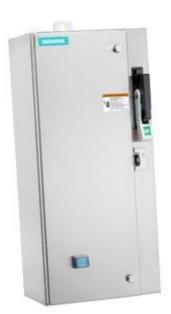
Non-reversing motor starter Size 0 Three phase full voltage Solidstate overload relay OLRelay amp range 0.25-1A 208VAC 60HZ coil Combination type 30Amp fusible disconnect 30Amp / 250V fuse clip Encl NEMA type 4X 316 S-steel Water/dust tight non-corrosive Standard width enclosure
