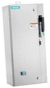
Non-reversing motor starter Size 0 Three phase full voltage Solidstate overload relay OLRelay amp range 0.25-1A 110VAC 50HZ / 120VAC 60HZ coil Combination type 30Amp fusible disconnect 30 Amp /600V fuse clip Encl NEMA type 4X 316 S-steel Water/dust tight non-corrosive Standard width enclosure
