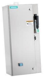
Non-reversing motor starter Size 0 Three phase full voltage Solidstate overload relay OLRelay amp range 0.25-1A 110VAC 50HZ / 120VAC 60HZ coil Combination type 30Amp non-fusible disconnect Encl NEMA type 4X 316 S-steel Water/dust tight non-corrosive Standard width enclosure
