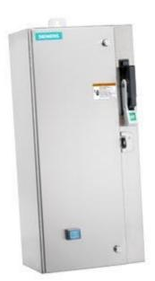
Non-reversing motor starter Size 0 Three phase full voltage Solidstate overload relay OLRelay amp range 0.25-1A Combination type 30Amp fusible disconnect 30Amp / 250V fuse clip Encl NEMA type 4X 316 S-steel Water/dust tight non-corrosive Standard width enclosure
