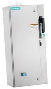
Non-reversing motor starter Size 0 Three phase full voltage Solidstate overload relay OLRelay amp range 0.25-1A Combination type 30Amp non-fusible disconnect Encl NEMA type 4X 316 S-steel Water/dust tight non-corrosive Standard width enclosure
