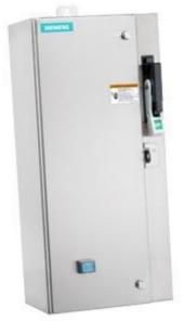
Non-reversing motor starter Size 0 Three phase full voltage Solidstate overload relay OLRelay amp range 0.25-1A 24VAC 50-60HZ coil Combination type 30Amp non-fusible disconnect Encl NEMA type 4X 316 S-steel Water/dust tight non-corrosive Standard width enclosure
