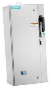
Non-reversing motor starter Size 0 Three phase full voltage Solidstate overload relay OLRelay amp range 0.25-1A 240VAC 50HZ / 277VAC 60HZ coil Combination type 30Amp fusible disconnect 30Amp / 250V fuse clip Encl NEMA type 4X 316 S-steel Water/dust tight non-corrosive Standard width enclosure
