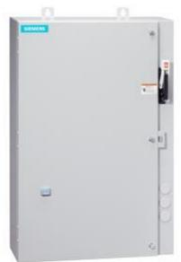
Non-reversing motor starter Size 0 Three phase full voltage Solidstate overload relay OLRelay amp range 0.75-3.4A 24Vdc coil Combination type 30Amp fusible disconnect 30Amp / 250V fuse clip Enclosure NEMA type 4/12 Water/dust tight weather proof Extra-wide enclosure
