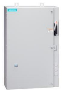
Non-reversing motor starter Size 0 Three phase full voltage Solidstate overload relay OLRelay amp range 0.75-3.4A 24Vdc coil Combination type 30Amp non-fusible disconnect Enclosure NEMA type 4/12 Water/dust tight weather proof Extra-wide enclosure
