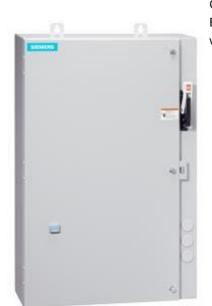
Non-reversing motor starter Size 0 Three phase full voltage Solidstate overload relay OLRelay amp range 0.75-3.4A 24Vdc coil Combination type 30Amp fusible disconnect 30 Amp /600V fuse clip Encl NEMA type 4X 304 S-steel Water/dust tight non-corrosive Extrawide enclosure
