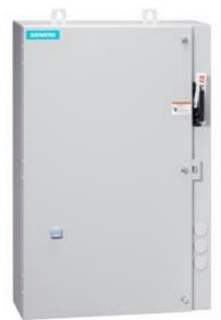
Non-reversing motor starter Size 0 Three phase full voltage Solidstate overload relay OLRelay amp range 0.75-3.4A 24Vdc coil Combination type 30Amp non-fusible disconnect Encl NEMA type 4X 304 S-steel Water/dust tight non-corrosive Extra-wide enclosure
