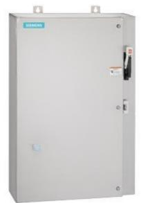
Non-reversing motor starter Size 0 Three phase full voltage Solidstate overload relay OLRelay amp range 0.75-3.4A Combination type 30Amp non-fusible disconnect Encl NEMA type 4X 316 S-steel Water/dust tight non-corrosive Extra-wide enclosure
