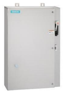
Non-reversing motor starter Size 0 Three phase full voltage Solidstate overload relay OLRelay amp range 0.75-3.4A Combination type 30Amp fusible disconnect 30Amp / 250V fuse clip Encl NEMA type 4X 316 S-steel Water/dust tight non-corrosive Extra-wide enclosure
