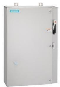
Non-reversing motor starter Size 0 Three phase full voltage Solidstate overload relay OLRelay amp range 0.75-3.4A Combination type 30Amp fusible disconnect 30 Amp /600V fuse clip Encl NEMA type 4X 316 S-steel Water/dust tight non-corrosive Extra-wide enclosure
