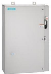
Non-reversing motor starter Size 0 Three phase full voltage Solidstate overload relay OLRelay amp range 0.75-3.4A 24VAC 50-60HZ coil Combination type 30Amp fusible disconnect 30Amp / 250V fuse clip Encl NEMA type 4X 316 S-steel Water/dust tight non-corrosive Extra-wide enclosure
