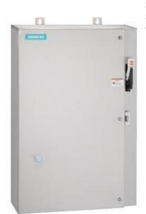
Non-reversing motor starter Size 0 Three phase full voltage Solidstate overload relay OLRelay amp range 0.75-3.4A 240VAC 50HZ / 277VAC 60HZ coil Combination type 30Amp fusible disconnect 30Amp / 250V fuse clip Encl NEMA type 4X 316 S-steel Water/dust tight non-corrosive Extra-wide enclosure
