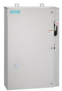
Non-reversing motor starter Size 0 Three phase full voltage Solidstate overload relay OLRelay amp range 0.75-3.4A 24Vdc coil Combination type 30Amp non-fusible disconnect Encl NEMA type 4X 316 S-steel Water/dust tight non-corrosive Extra-wide enclosure
