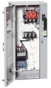
Non-reversing motor starter Size 0 Three phase full voltage Solidstate overload relay OLRelay amp range 0.75-3.4A 24Vdc coil Combination type 30Amp fusible disconnect 30 Amp /600V fuse clip Enclosure NEMA type 1 Indoor general purpose use Standard width enclosure
