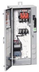
Non-reversing motor starter Size 0 Three phase full voltage Solidstate overload relay OLRelay amp range 0.75-3.4A 24Vdc coil Combination type 30Amp fusible disconnect 30Amp / 250V fuse clip Enclosure NEMA type 4/12 Water/dust tight weather proof Standard width enclosure
