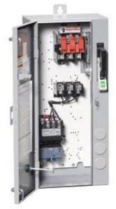
Non-reversing motor starter Size 0 Three phase full voltage Solidstate overload relay OLRelay amp range 0.75-3.4A 24Vdc coil Combination type 30Amp fusible disconnect 30 Amp /600V fuse clip Enclosure NEMA type 4/12 Water/dust tight weather proof Standard width enclosure
