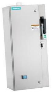
Non-reversing motor starter Size 0 Three phase full voltage Solidstate overload relay OLRelay amp range 0.75-3.4A 24Vdc coil Combination type 30Amp fusible disconnect 30Amp / 250V fuse clip Encl NEMA type 4X 304 S-steel Water/dust tight non-corrosive Standard width enclosure
