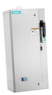
Non-reversing motor starter Size 0 Three phase full voltage Solidstate overload relay OLRelay amp range 0.75-3.4A Combination type 30Amp fusible disconnect 30Amp / 250V fuse clip Encl NEMA type 4X 316 S-steel Water/dust tight non-corrosive Standard width enclosure
