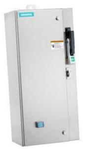
Non-reversing motor starter Size 0 Three phase full voltage Solidstate overload relay OLRelay amp range 0.75-3.4A 208VAC 60HZ coil Combination type 30Amp non-fusible disconnect Encl NEMA type 4X 316 S-steel Water/dust tight non-corrosive Standard width enclosure
