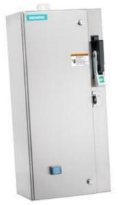
Non-reversing motor starter, Size 0, Three phase full voltage, Solid-state overload relay, OLRelay amp range 0.75-3.4a, 110V 50HZ / 120V 60HZ coil, Combination type, 30Amp fusible disconnect 30 Amp /250V fuse clip, Encl NEMA type 4X 316 S-steel Water/dust tight noncorrosive, Standard width enclosure
