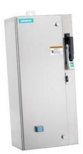
Non-reversing motor starter Size 0 Three phase full voltage Solidstate overload relay OLRelay amp range 0.75-3.4A 110VAC 50HZ / 120VAC 60HZ coil Combination type 30Amp non-fusible disconnect Encl NEMA type 4X 316 S-steel Water/dust tight non-corrosive Standard width enclosure
