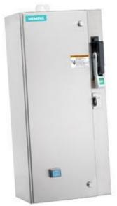
Non-reversing motor starter Size 0 Three phase full voltage Solidstate overload relay OLRelay amp range 0.75-3.4A Combination type 30Amp non-fusible disconnect Encl NEMA type 4X 316 S-steel Water/dust tight non-corrosive Standard width enclosure
