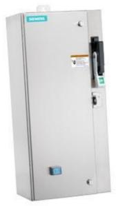
Non-reversing motor starter, Size 0, Three phase full voltage, Solidstate overload relay, OLRelay amp range 0.75-3.4a, 380 440/440 480V 50/60HZ coil, Combination type, 30Amp fusible disconnect 30 Amp /600V fuse clip, Encl NEMA type 4X 316 S-steel Water/dust tight noncorrosive, Standard width enclosure
