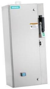
Non-reversing motor starter Size 0 Three phase full voltage Solidstate overload relay OLRelay amp range 0.75-3.4A 24VAC 50-60HZ coil Combination type 30Amp fusible disconnect 30Amp / 250V fuse clip Encl NEMA type 4X 316 S-steel Water/dust tight non-corrosive Standard width enclosure
