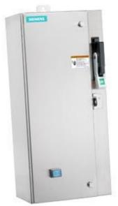
Non-reversing motor starter Size 0 Three phase full voltage Solidstate overload relay OLRelay amp range 0.75-3.4A 24Vdc coil Combination type 30Amp fusible disconnect 30Amp / 250V fuse clip Encl NEMA type 4X 316 S-steel Water/dust tight non-corrosive Standard width enclosure
