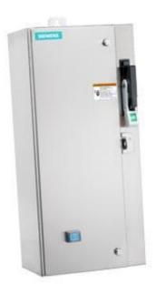
Non-reversing motor starter Size 0 Three phase full voltage Solidstate overload relay OLRelay amp range 0.75-3.4A 24Vdc coil Combination type 30Amp fusible disconnect 30 Amp /600V fuse clip Encl NEMA type 4X 316 S-steel Water/dust tight non-corrosive Standard width enclosure
