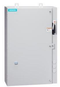
Non-reversing motor starter Size 0 Three phase full voltage Solidstate overload relay OLRelay amp range 3-12A 24Vdc coil Combination type 30Amp non-fusible disconnect Enclosure NEMA type 4/12 Water/dust tight weather proof Extra-wide enclosure
