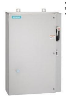
Non-reversing motor starter Size 0 Three phase full voltage Solidstate overload relay OLRelay amp range 3-12A 24VAC 50-60HZ coil Combination type 30Amp fusible disconnect 30Amp / 250V fuse clip Encl NEMA type 4X 316 S-steel Water/dust tight non-corrosive Extrawide enclosure
