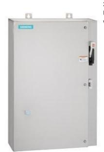
Non-reversing motor starter Size 0 Three phase full voltage Solidstate overload relay OLRelay amp range 3-12A 240VAC 50HZ / 277VAC 60HZ coil Combination type 30Amp non-fusible disconnect Encl NEMA type 4X 316 S-steel Water/dust tight non-corrosive Extrawide enclosure
