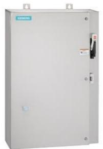
Non-reversing motor starter Size 0 Three phase full voltage Solidstate overload relay OLRelay amp range 3-12A 24Vdc coil Combination type 30Amp fusible disconnect 30Amp / 250V fuse clip Encl NEMA type 4X 316 S-steel Water/dust tight non-corrosive Extrawide enclosure
