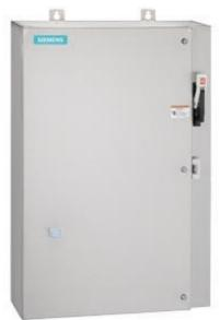
Non-reversing motor starter Size 0 Three phase full voltage Solidstate overload relay OLRelay amp range 3-12A 24Vdc coil Combination type 30Amp fusible disconnect 30 Amp /600V fuse clip Encl NEMA type 4X 316 S-steel Water/dust tight non-corrosive Extrawide enclosure
