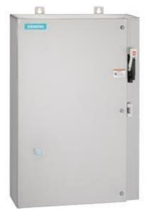
Non-reversing motor starter Size 0 Three phase full voltage Solidstate overload relay OLRelay amp range 3-12A 24Vdc coil Combination type 30Amp non-fusible disconnect Encl NEMA type 4X 316 S-steel Water/dust tight non-corrosive Extra-wide enclosure
