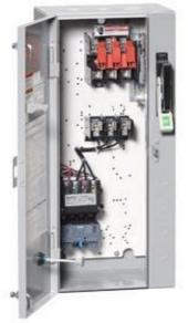
Non-reversing motor starter Size 0 Three phase full voltage Solidstate overload relay OLRelay amp range 3-12A 24VAC 50-60HZ coil Combination type 30Amp fusible disconnect 30 Amp /600V fuse clip Enclosure NEMA type 1 Indoor general purpose use Standard width enclosure
