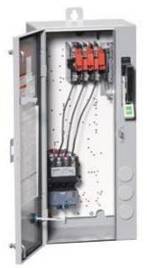
Non-reversing motor starter, Size 0, Three phase full voltage, Solid-state overload relay, OLRelay amp range 3-12a, 110V 50HZ / 120V 60HZ coil, Combination type, 30Amp non-fusible disconnect Enclosure NEMA type 4/12, Water/dust tight for outdoors, Standard width enclosure
