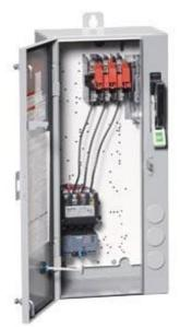
Non-reversing motor starter, Size 0, Three phase full voltage, Solid-state overload relay, OLRelay amp range 3-12a, 190 220/220 240V 50/60HZ coil, Combination type, 30Amp non-fusible disconnect Enclosure NEMA type 4/12, Water/dust tight for outdoors, Standard width enclosure
